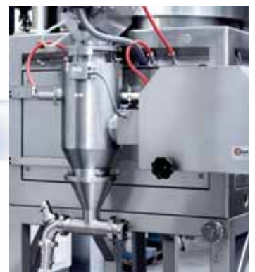
Product discharge with attached Glatt wet sieve GSF 180 with suction shoe for pneumatical product transfer
