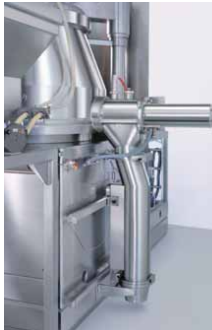
Product discharge with docked bypass pipe alternative to the wet sieve
