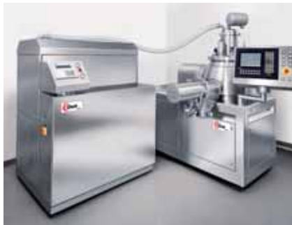
Vertical granulator VG 100 with solvent recovery / solvent separation
